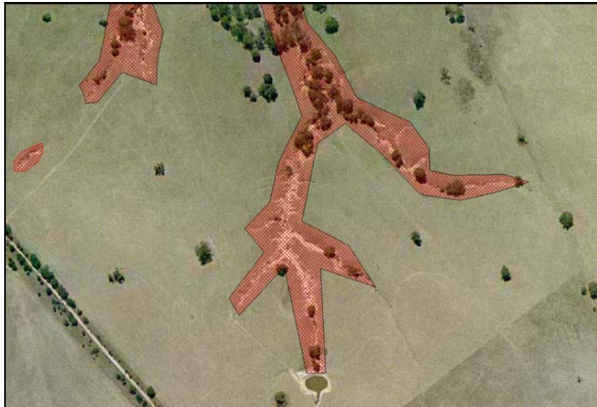
Figure 3.3 . Feature WF58. Aerial Photo Mapping of gully erosion with polygon object overlying the erosion feature.
