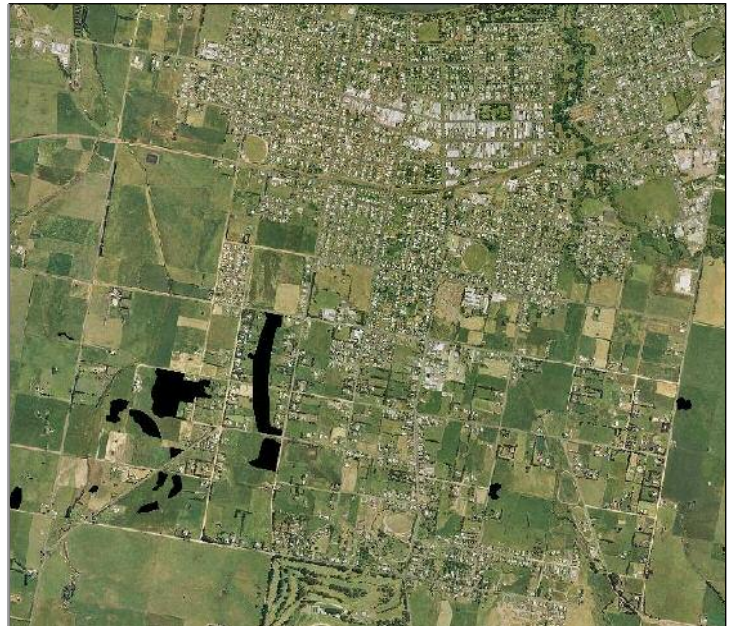
Figure 3.4: Salinity encroaching into the City of Colac (Salinity is shown by the black polygons)
