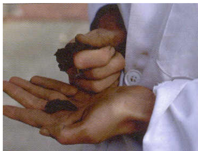
Figure 1: Using the 'ribbon' technique to determine soil texture
