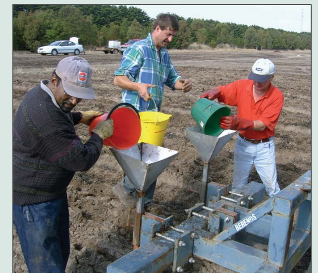
Slotting the soil with a slurry of poultry manure. Picture shows the laborious calibration operation.
