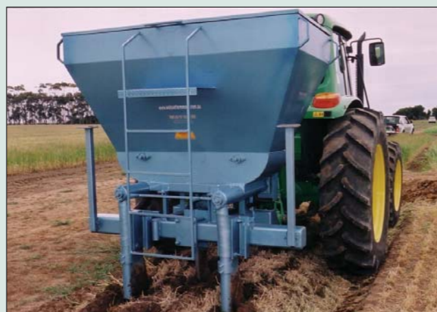
The 'modified' deep ripper that was used in small plot trials to incorporate organic substances to the subsoil at the time of deep ripping
