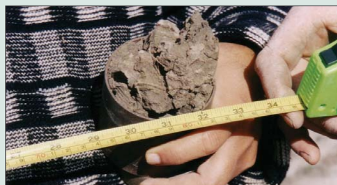
Intact soil core taken from 80cm depth in a 4-year lucerne paddock showing the intensity of cracking
