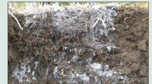
Paint percolation study showing friable topsoil overlying the heavy clay, where the paint simply followed preferential pathways (cracks).
