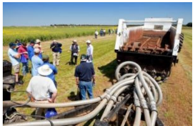
This commercial machine, recently developed by the Geelong Director of SFS John Sheehan, is capable of manuring one hectare of land in one fill and has six rippers which cover a width of six metres.
