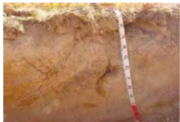
6d Soil pit in plot F showing average depth of tunnel erosion in the paddock
