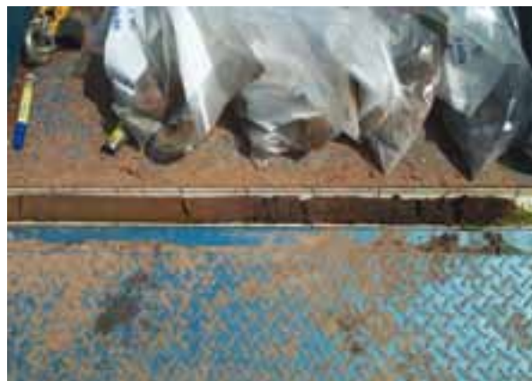
Figure 10: The Intact corer at work (left) and the core sample from plot C showing the sandy subsoil (right).
