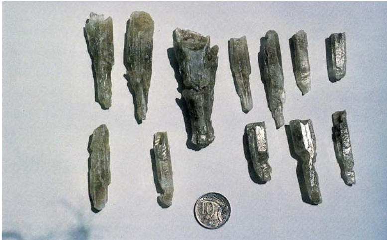
Figure 9.16 – Prismatic selenite crystals
