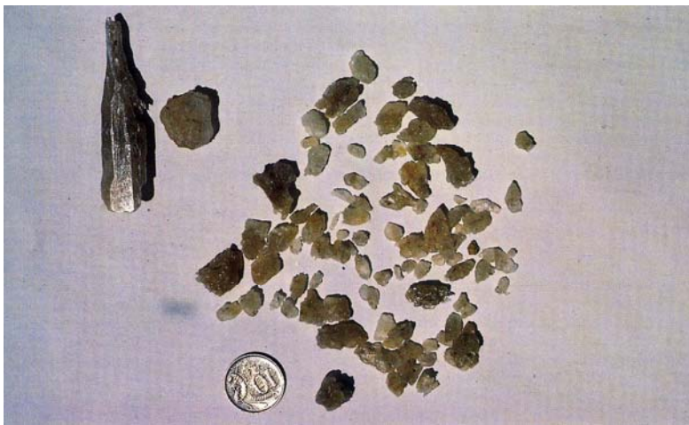
Figure 9.17 - Stubby and irregular gypsum, precipitated from groundwater in the zone of overlapping spring and lake waters lakeward of that shown in Figure 9.15. The loss of prismatic morphology reflects the rising pH under the influence of the neutral pH lake regime.
