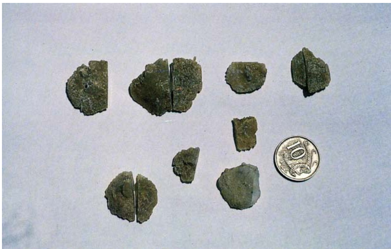
Figure 9.14 - Discoidal gypsum precipitated in near surface sediments from inflowing groundwaters within the spring zone (diameter of the coin is 24 mm).
