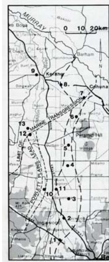
Figure 4.6a - Piezometer network in the Loddon Valley
