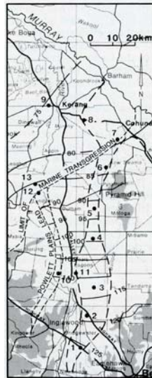
Figure 4.6b - Potentiometric surface - Calivil Formation and Parilla Sand
